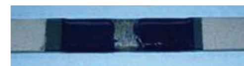
Distension reduced failure picture of enamel in the bending test in the area of the plastic deformation (load transmission). Outside of the plastic zone, left and right, damage-free enamel.
