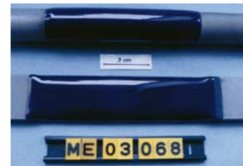
Outer glass lined pipe probe DN15 (1/2") for the tensile test (top). Onesided glass lined flat probe for the three-point bending test (bottom)
